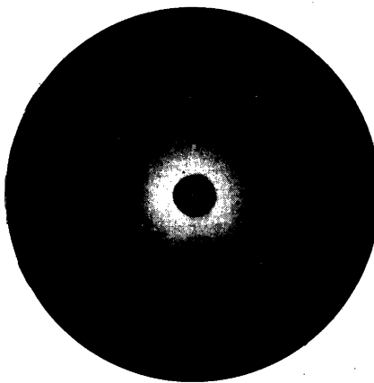
Fig. 7. X-ray diffraction diagram of charcoal-sulphur compound (approx. 13 % S). The preparation has been heated and then extracted with carbon disulphide.
